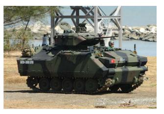
The AIFV is fitted with a stabilised 25 mm manned or remote-controlled SABER turret and can carry 11 personnel including driver, commander and gunner.
