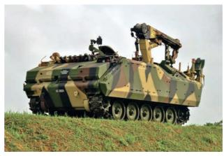
The ARV variant is the Armoured Recovery Vehicle configuration of the ACV-15 FoV. It is fitted with a hydraulic crane mounted on the vehicle's top plate and a hydraulic recovery winch with a fairlead assembly mounted inside the vehicle, which facilitates the recovery and towing of both armoured and non-armoured vehicles in difficult terrains. It is armed with a self-defence 12.7 mm MG and can carry 4 personnel including driver, gunner, and 2 technicians.
